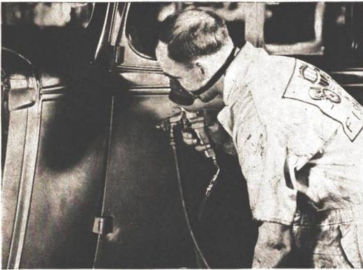
**1** They thoroughly wash each new Fisher Body with an acid solution to remove all the dust and grease. Then, in a special booth, they spray on the "priming coat." After baking in an oven, the body moves on to another booth for a "glaze" coat—which is also baked on.
